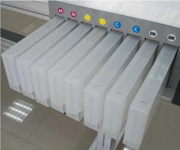
2.7.2 Remove rubber cap on each cartridge, fill the ink in to the cartridge by using funnel. Please make sure the ink color should be match with the marks on the cartridge.
