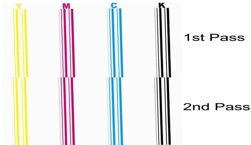
Loose three head fixing screws, turn head adjust screw slightly, print again until the
