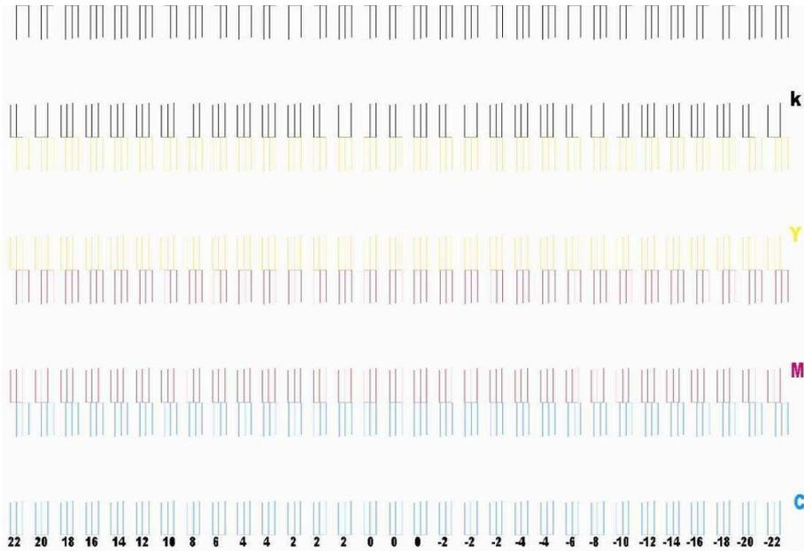
Look at the chart printed, find the each line of individual color that is most matching black line, the value under the line is the deviation to be filled in related color.
