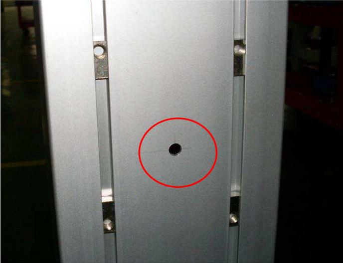
Fixing the beam by 4 pcs of M6X16 Hex screws, see below fig:
