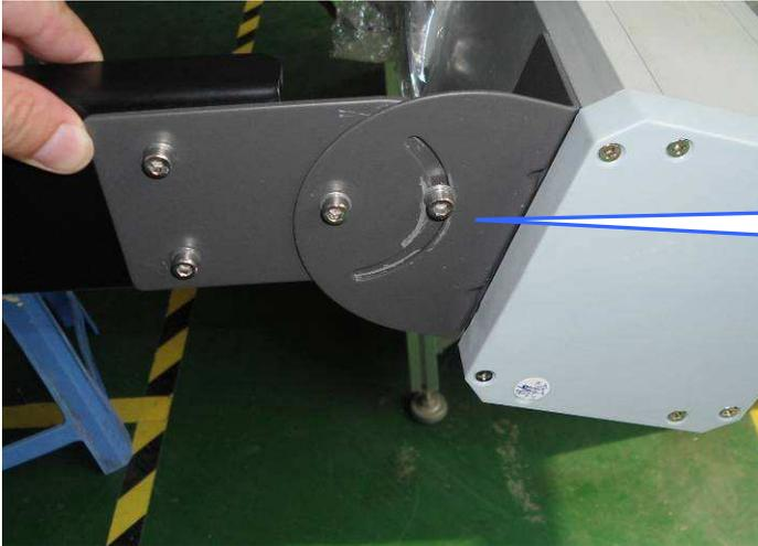
Turn the drier to proper angle.
