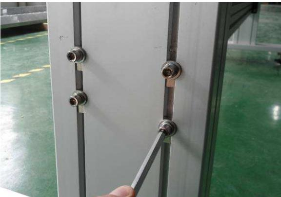
Install the bracket. Make sure two brackets in both side are in the same level.
