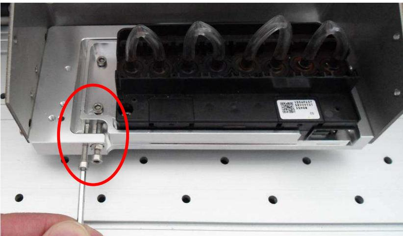
**Note:** The screws are used to adjust the straightness of the head.
