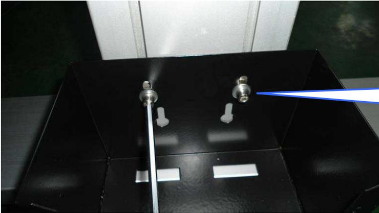
Push the holder down to the end and fix it by two M8X14 Hex screws.
