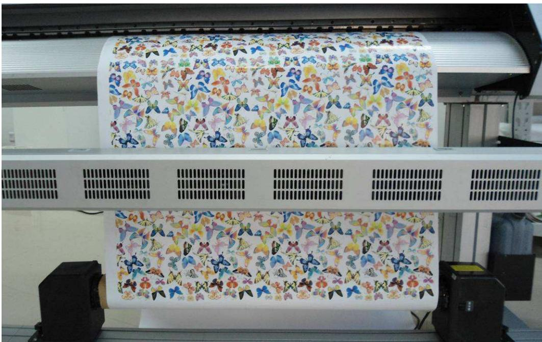
7.3.3 Switch on take up system, select winding direction.
