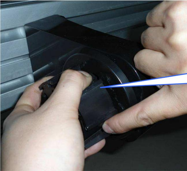
Push the clips in for position, remove 3 in core adaptor.
