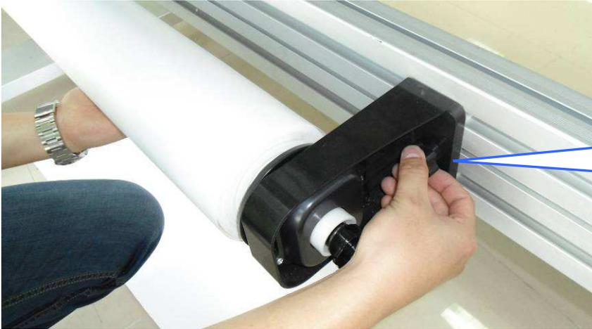
Push the holder then fasten the fixing screw.
