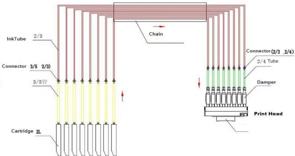
Fig 5-1 Clean System Diagram
