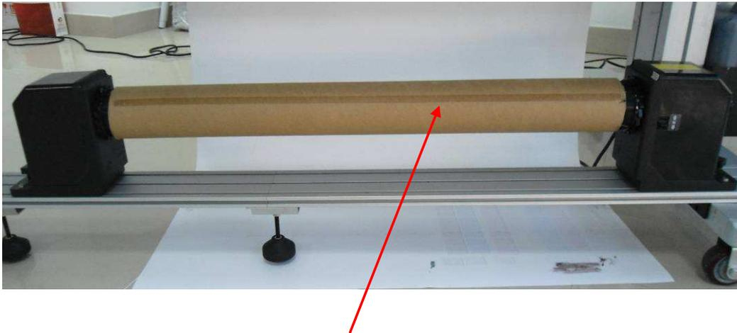
Install paper core, stick a double side adhesive in horizontal on the surface of the paper core.
