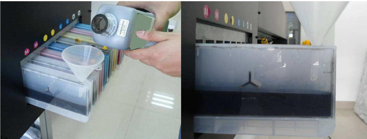
2.7.3 Connect the injector with the damper, draw the ink out from the cartridge into the damper.
