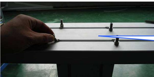
Fixing the leg and the pillar with the 4 screws removed.
