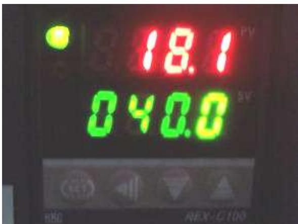
Step 2: Press shift key, Lighten the digit to be changed.
