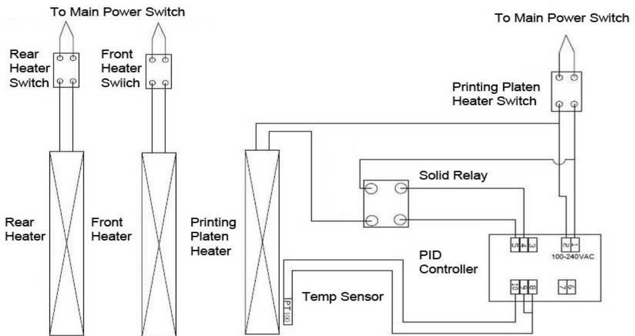
Fig 6-1 Heating System Diagram
