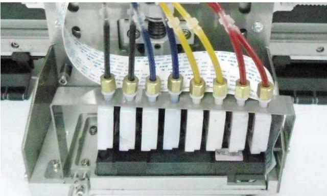
2.7.5 Install and fix damper holder after all dampers are connected with the head correctly.
