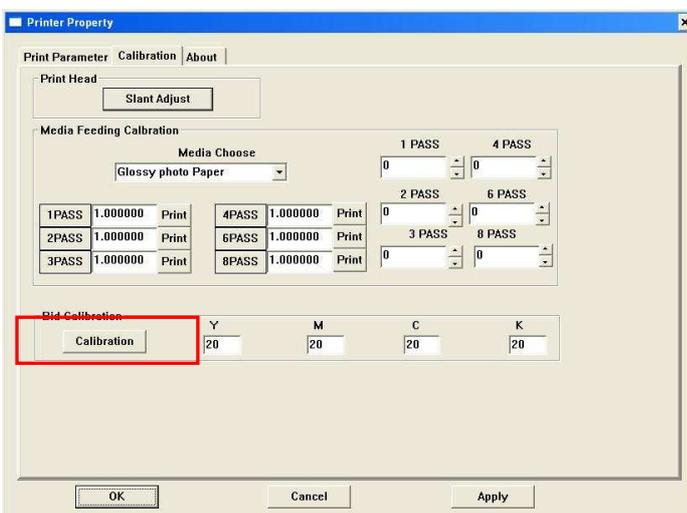
Click “Calibration” on Bid calibration, the printer will print the checking chart as below:
