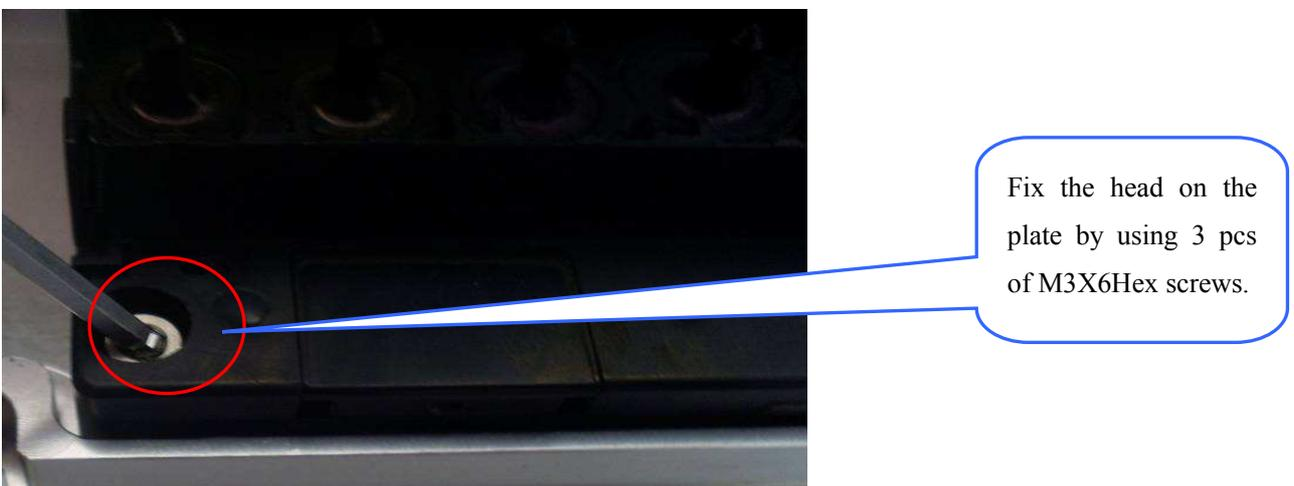
2.6.3 put the head assembly on the carriage and fix it by 3 pcs of M#X6 Hex screws on head plate.
